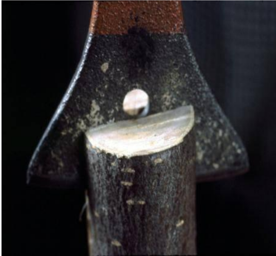
Close up photo showing a wedge splitting a stub.
