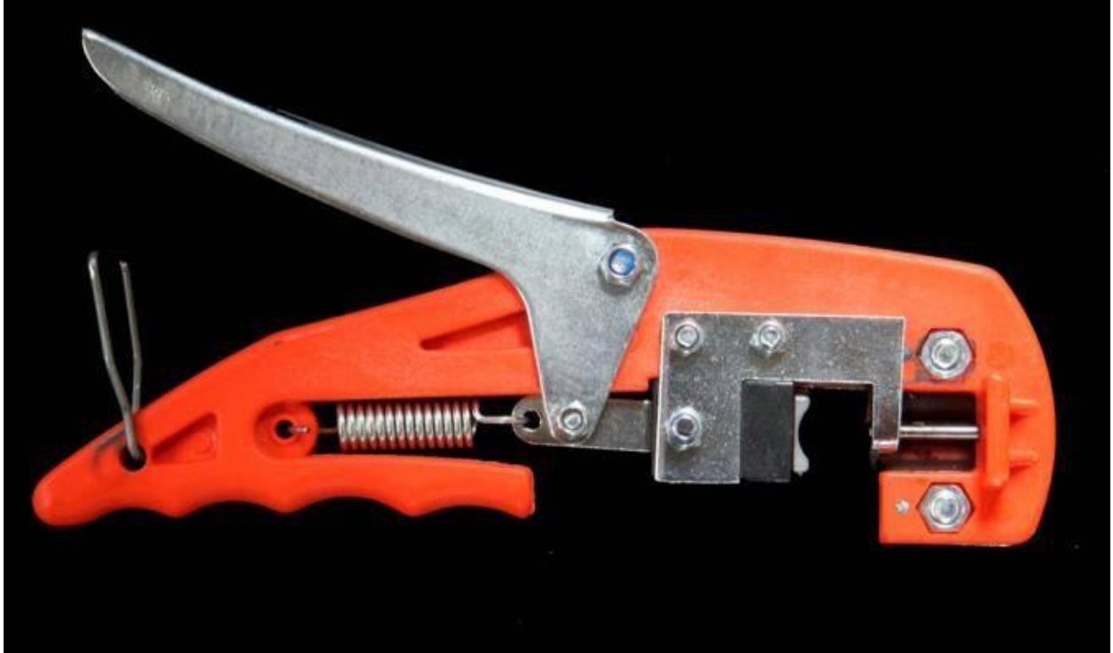
Photo of a hand held grafting machine.
