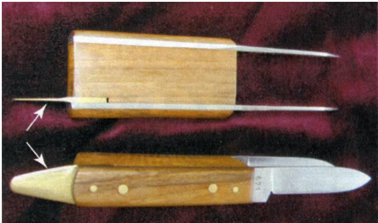
Photo showing a tool with two parallel knife blades to create consistently sized cuts for patch budding.
