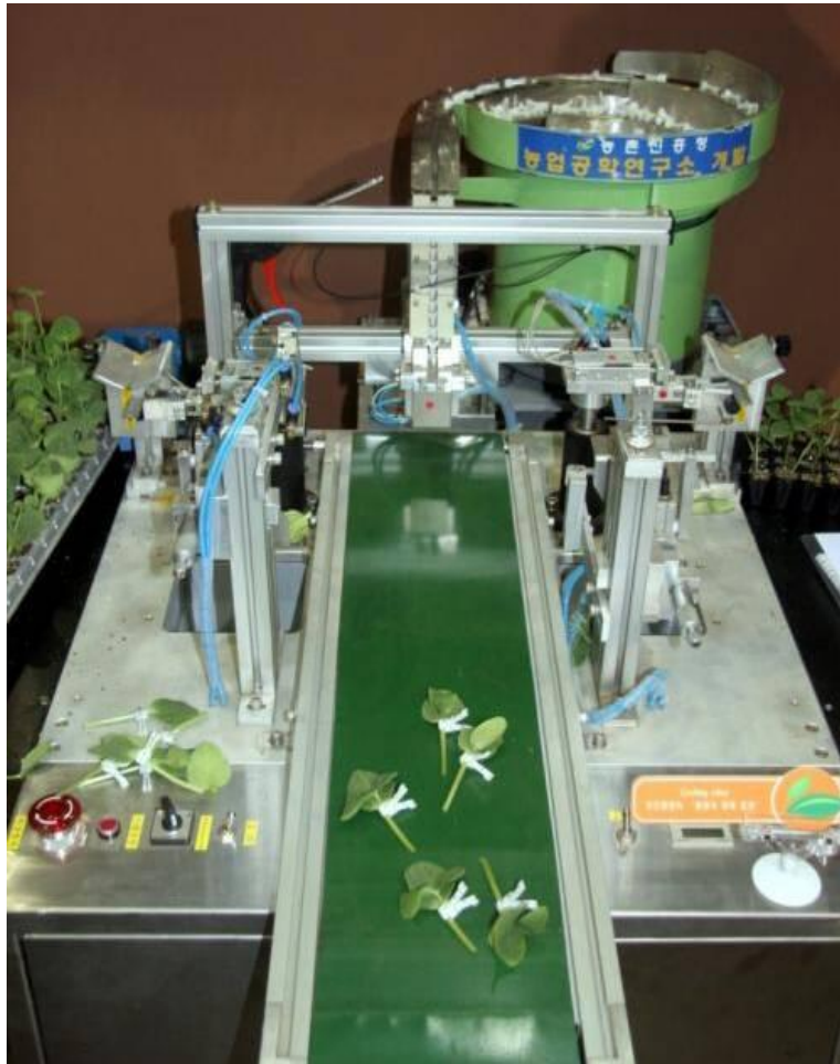
Photo of robotic grafting machine.
